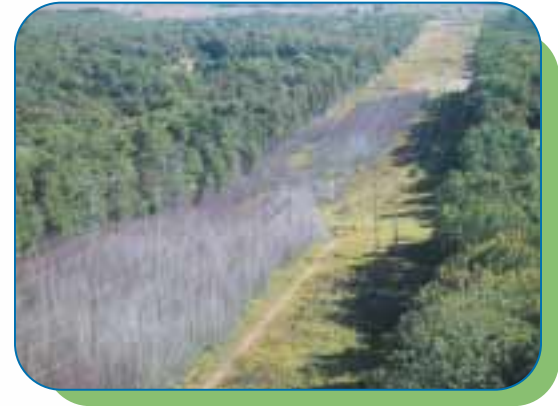
Deferring maintenance threatens reliability and can obstruct access, whereas conducting vegetation management allows you to manage to a stable plant community and decrease maintenance costs over time.
