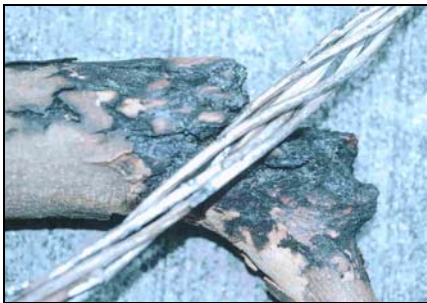
Tree limb burned by contact with utility wires Removal of limbs that have fallen on lines.
